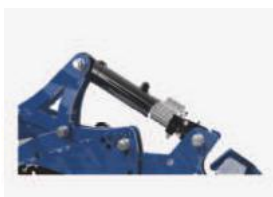
Hydraulic adjustment of working depth - OPTION
