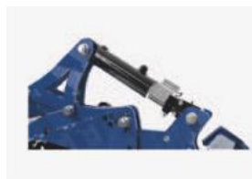
Hydraulic adjustment of working depth - OPTION
