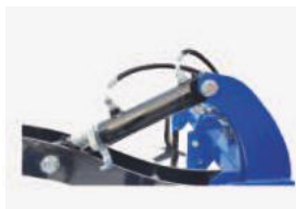
Hydraulic adjustment of working depth - OPTION
