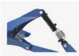
Hydraulic adjustment of working depth - STANDARD
