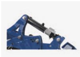
Hydraulic adjustment of working depth - OPTION
