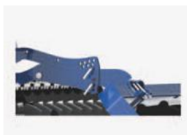
Hydraulic adjustment of working depth - STANDARD
