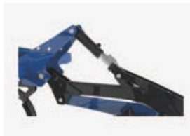
Hydraulic adjustment of working depth - STANDARD
