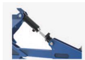
Hydraulic adjustment of working depth - STANDARD
