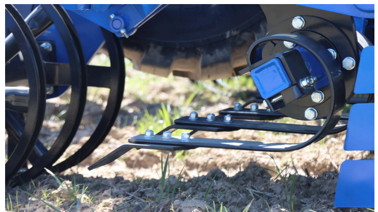
Crushboard – in front of the roller (hydraulic adjustment)
