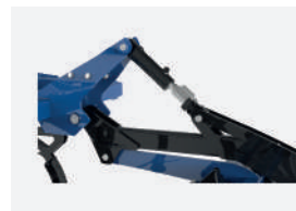
Hydraulic adjustment of working depth - STANDARD
