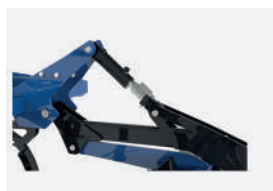
Hydraulic adjustment of working depth – OPTION
