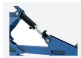
Hydraulic adjustment of working depth - STANDARD
