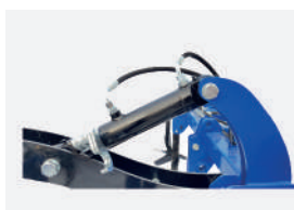
Hydraulic adjustment of working depth - OPTION
