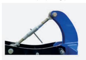
Adjustment of working depth - STANDARD
