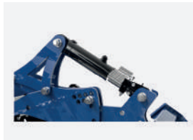
Hydraulic adjustment of working depth - OPCJA
