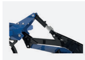
Hydraulic adjustment of working depth - STANDARD
